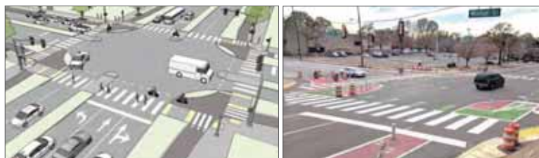
Exhibit 19. Protected Intersection Design Concept (see Appendix B ) with Example from Memphis, TN of using low-cost and removable materials (Right)
